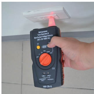
Detect voltage in wall outlet
